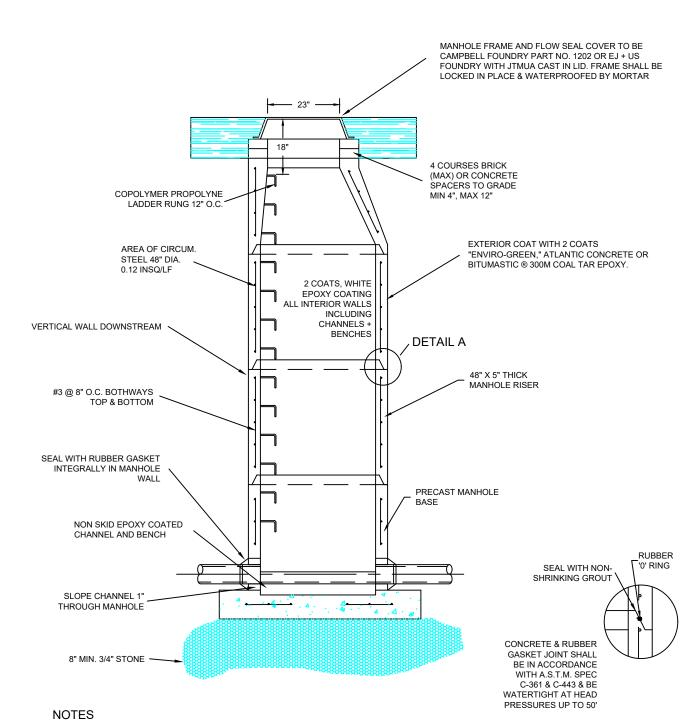
1. THE CONTRACTOR SHALL BE RESPONSIBLE FOR CONSTRUCTING ADEQUATE BALLASTS TO OFFSET FLOTATION FORCES ACTING ON MANHOLES 2. ALL REINFORCEMENT IS SUBJECT TO **ENGINEERS APPROVAL BEFORE CONSTRUCTION**
