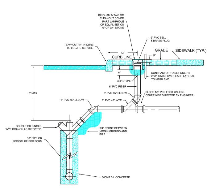
NOTE: LOCATION OF SERVICE CONNECTION & CLEANOUT SHALL BE DETERMINED IN THE FIELD TO COMPLY WITH REQUIREMENTS OF THE PROPERTY OWNER & M.U.A. CLEAN-OUT IS NOT PERMITTED IN DRIVEWAY OR SIDEWALK. IT SHALL BE INSTALLED BETWEEN THE CURB AND THE SIDEWALK. SHOULD NO CURBING EXIST A 2' X 2' X 6" CONCRETE COLLAR IS REQUIRED TO BE CONSTRUCTED.
