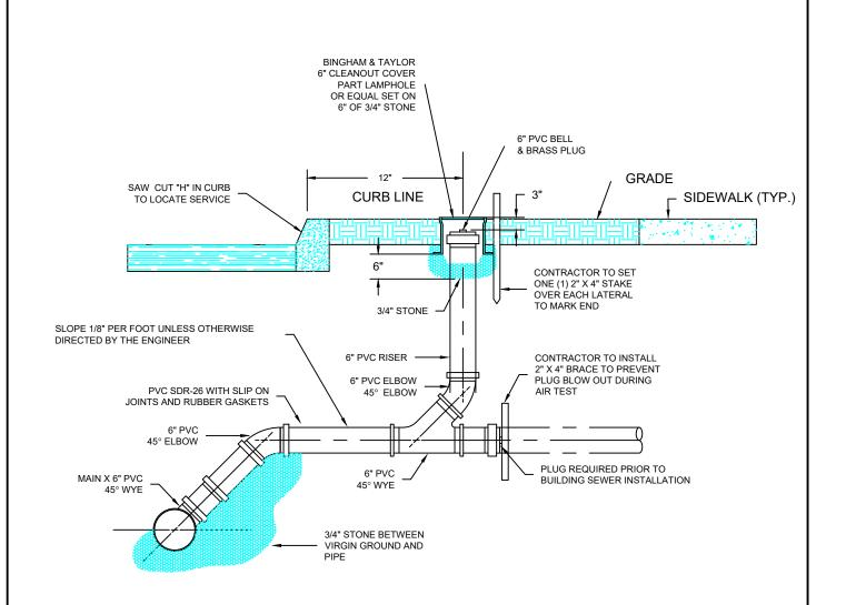
NOTE: LOCATION OF SERVICE CONNECTION & CLEANOUT SHALL BE DETERMINED IN THE FIELD TO COMPLY WITH REQUIREMENTS OF THE PROPERTY OWNER & M.U.A. CLEAN-OUT IS NOT PERMITTED IN DRIVEWAY OR SIDEWALK. IT SHALL BE INSTALLED BETWEEN THE CURB AND THE SIDEWALK. SHOULD NO CURBING EXIST A 2' X 2' X 6" CONCRETE COLLAR IS REQUIRED TO BE CONSTRUCTED.
