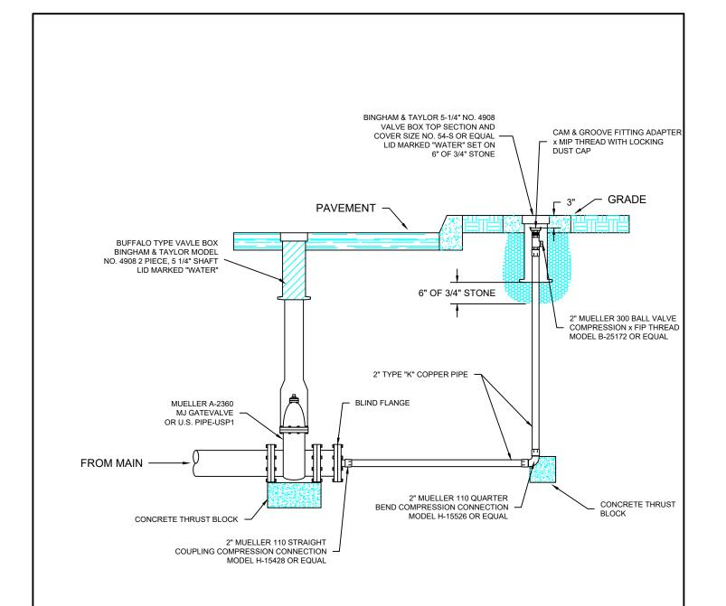
1. ANY VALVE INSTALLED OUTSIDE OF ASPHALT AREAS MUST BE CONSTRUCTED WITH AN 18" PRE-FORMED SONO TUBE, CONCRETE COLLAR AROUND IT.
